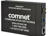
The ComNet CWGE2SFP Ethernet media converter series are one-channel Ethernet electrical to optical media converters. These auto-negotiating devices accept a 10/100/1000 Mbps electrical input and convert this to a 1000 Mbps optical output. These devices use either one or two optical fibers, depending upon the selection of either included or sold-separately SFP\* optical module. These devices can be used in stand-alone mode or can be installed within the ComNet CWCHASSIS 19 inch rack.
